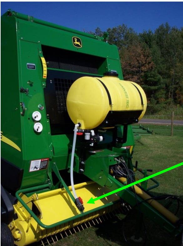
Drain/Fill line on the baler
