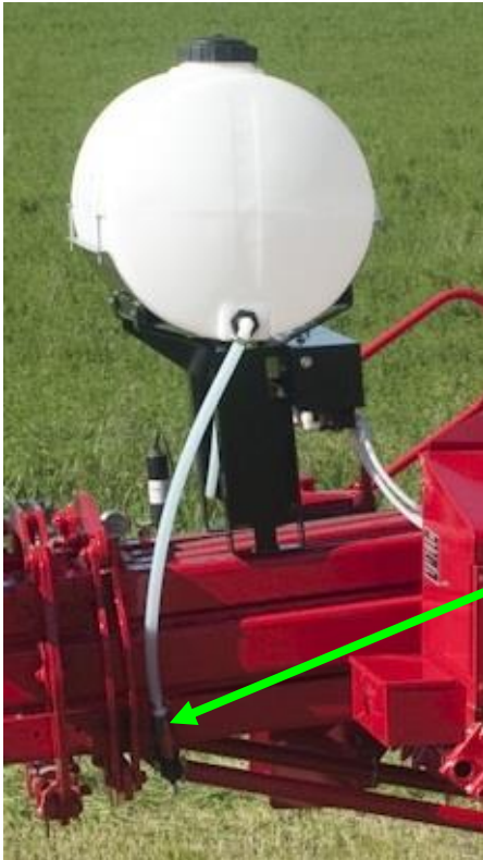
Drain/Fill line on the baler
