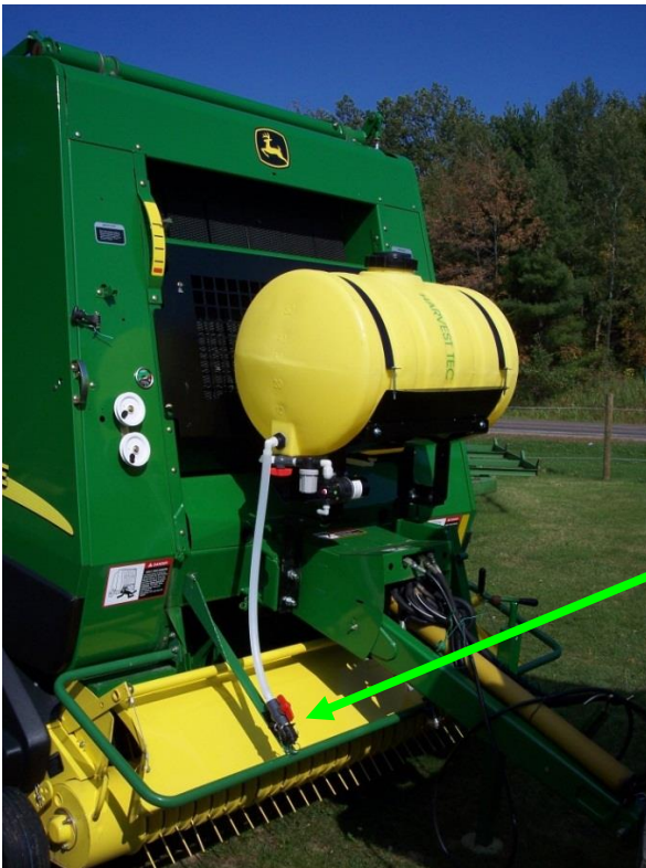
Drain/Fill line on the baler
