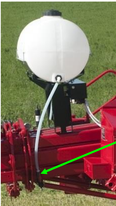
Drain/Fill line on the baler
