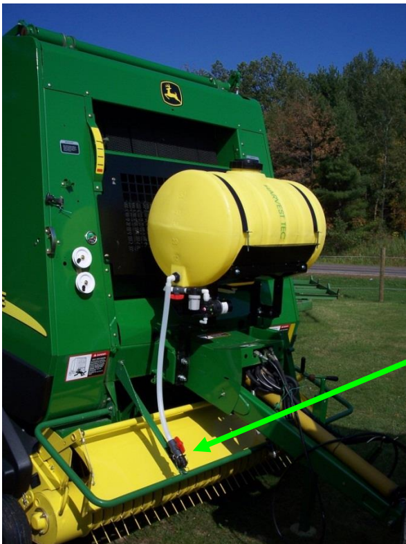
Drain/Fill line on the baler
