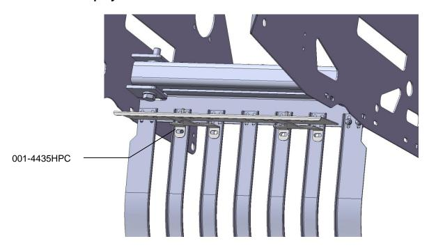
Mount the two spray shield mounting brackets (001-4435HPC) to the baler as shown above. Attach using four 3/8" x 1-1/4" bolts, flats, locks, and nuts. Mount the spray shield (001-4435ES) on top of the mounting brackets and secure with two lynch pins. Use the inside slots on 3x3 balers and outside slots on 3x4 and 4x4 balers.
