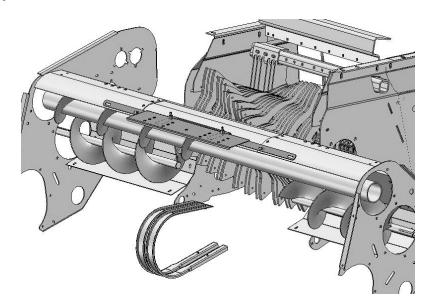
Locate bottom hole on each side of center insert over top auger and bolt spray shield and mounting bracket into place using the 3/8" x 1-1/4" carriage bolts, nuts, locks, and flat washers. Use the inside slots on 3x3 balers and the outside slots on 3x4 and 4x4 balers.
