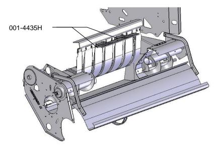
Remove the four bolts attached to the wrapper stripper plates as shown above. Replace with the four supplied 3/8" x 1-1/4" carriage bolts, nuts, locks, and flat washers. Mount the spray shield holders (001-4435H) and loosely tighten down hardware. Install spray shield and secure with the two supplied lynch pins. Tighten all hardware. Use the inside slots on 3x3 balers and the outside slots on 3x4 and 4x4 balers.
