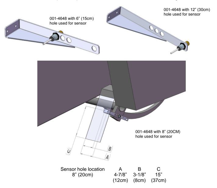
Mount the end of bale sensor bracket (001-4648) as shown in the 8" (20cm) hole position. Mark and drill two 3/8" (10mm) holes and attach the bracket using two 5/16" x 1" self-tapping screws, and 5/16" flange nuts. Mount the sensor in the 8" (20cm) hole location, keep the sensor 1/4" (7mm) from the needle arm and tighten both nuts. Cut off excess metal past the sensor. Run the sensor cable up to the Dual channel Processor (DCP) and secure to the baler.
