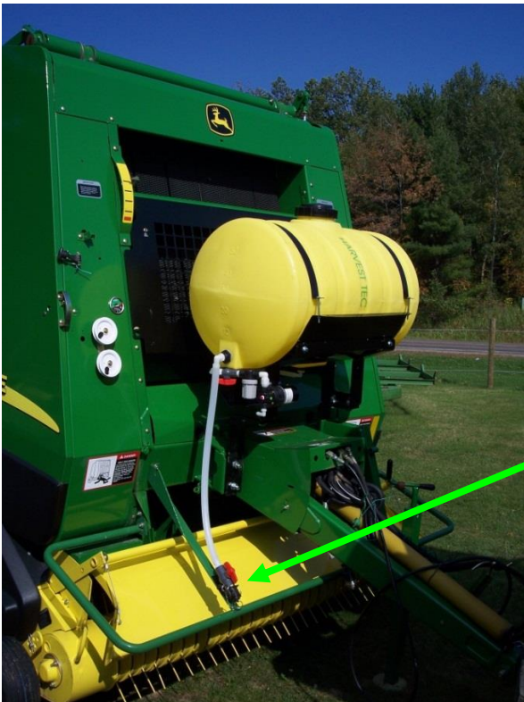
Drain/Fill line on the baler
