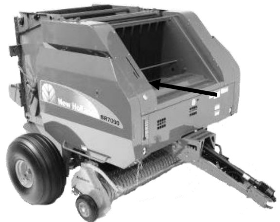
Mount THS on Left Side of Bale Chamber Panel Above Baler Shelf
