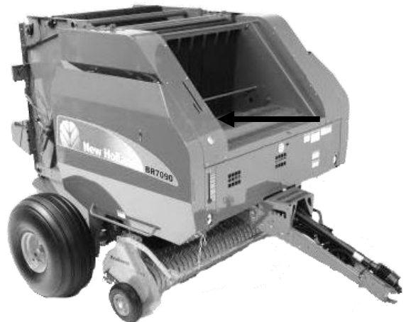
Mount DCP on Left Side of Bale Chamber Panel Above Baler Shelf
