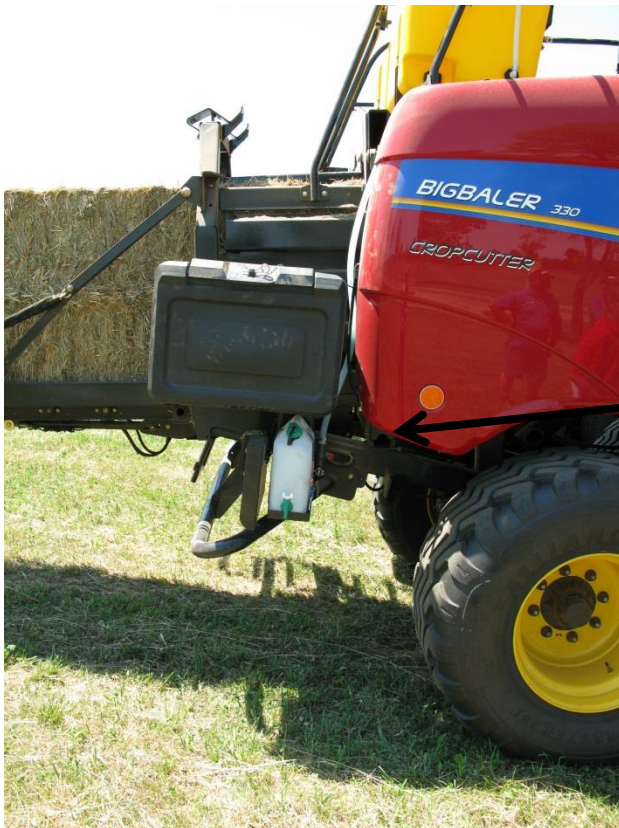
Drain/Fill line on right side of baler
