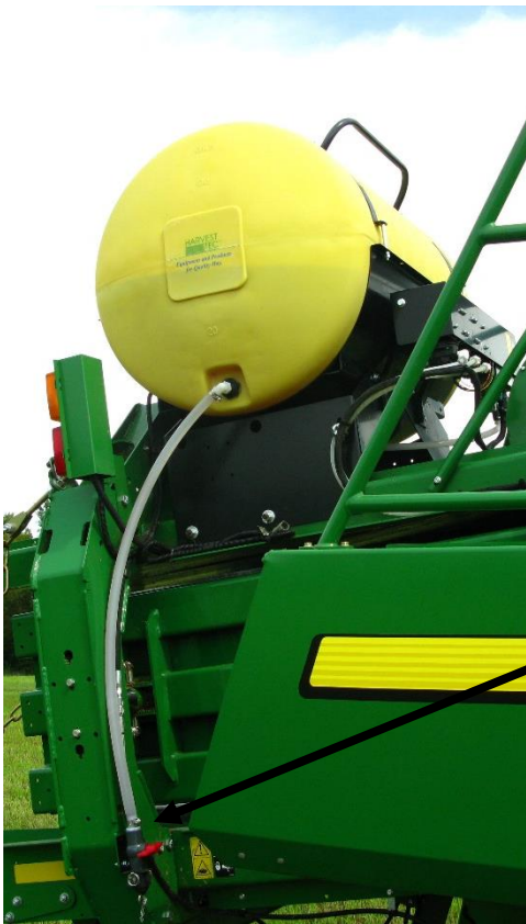
Drain/Fill line on right side of baler
