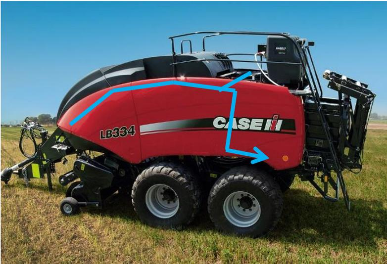
Route harnesses along inside of the baler (Left). Keep harnesses away from moving parts and hydraulic hoses. Secure with existing cable clamps or use cable ties.
