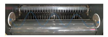
The moisture sensor has two discs in the bale chamber that read across the width of the bale, taking 5 readings of resistance per second, giving the operator complete visibility of crop conditions.
