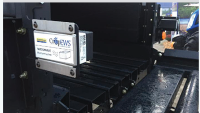
▲ Microwave sensors mounted on the rear of bale chamber
