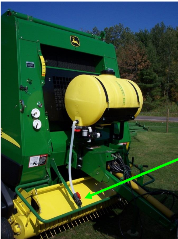
Drain/Fill line on the baler
