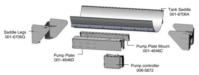
Locate parts bag 3. Install both saddle legs (001-6706Q) onto the saddle (001-6706A) with six 3/8" x 1-1/4" bolts, locks and flat washers. The mounting slots in the legs will attach to the second and third weld nuts in from each end, of the saddle, on both sides.
