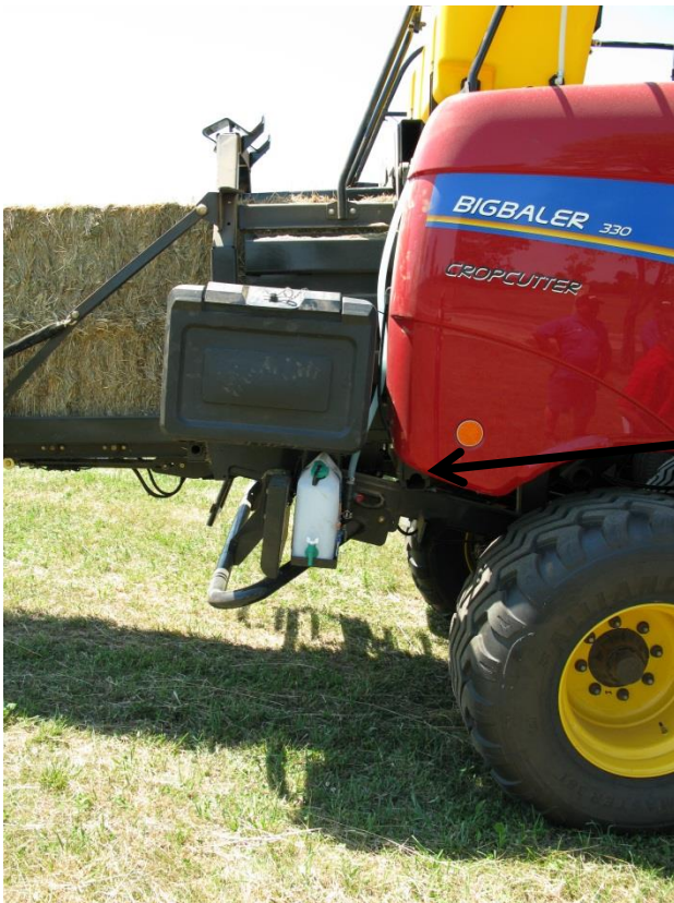
Drain/Fill line on right side of baler
