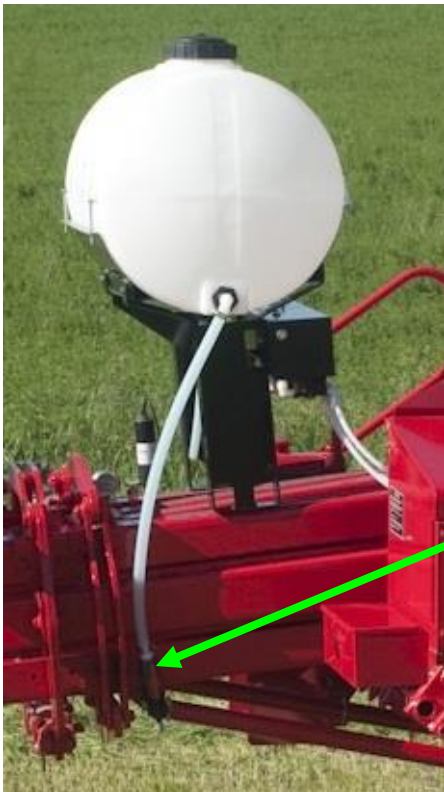
Drain/Fill line on the baler
