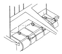
Bend the nozzle bars up so that the tip sprays in the generally horizontal direction and is pointed toward the intake rolls of the baler at the end of the pick-up head. The tips should be located so that they will be somewhere between 14" and 18" from the normal path of hay.
