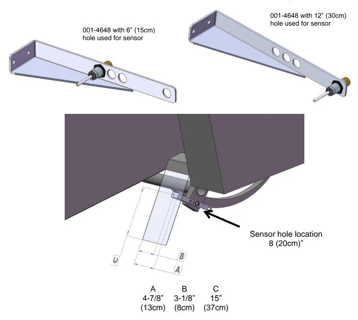
Mount the end of bale sensor bracket (001-4648) as shown. Mark and drill two 5/16" (8mm) holes and attach the bracket using two 1/4" x 1" bolts, locks, flats, and nuts. Mount the sensor in the 8" (20cm) hole location, keep the sensor 1/4" (7mm) from the needle and tighten both nuts. Cut off excess metal past the sensor. Run the sensor cable up to the Dual Channel Processor and secure to the baler.
