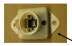
B. Under the chamber locate the Active Terminator from the end of the baler harness. It is located at the right rear corner of the baler frame. Attach Baler Interface Harness (006-6650VA) to that location. Reconnect Active Terminator to open port of that same harness (006-6650VA). If your baler does not have a Terminator at this location please call Harvest Tec.
