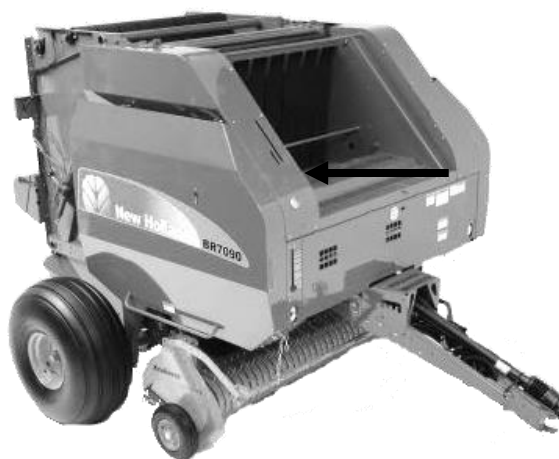
Mount DCP on Left Side of Bale Chamber Panel Above Baler Shelf
