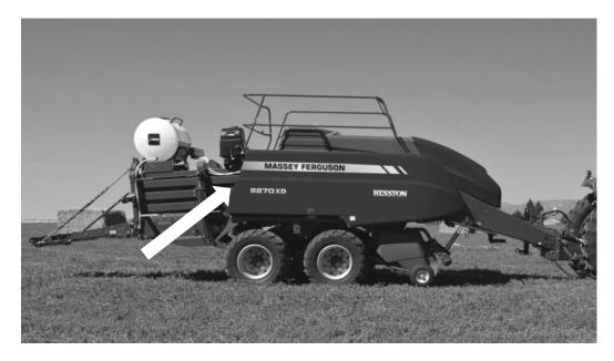
2. Insert Harvest Tec USB drive with RFV Software into USB port on DCP.
