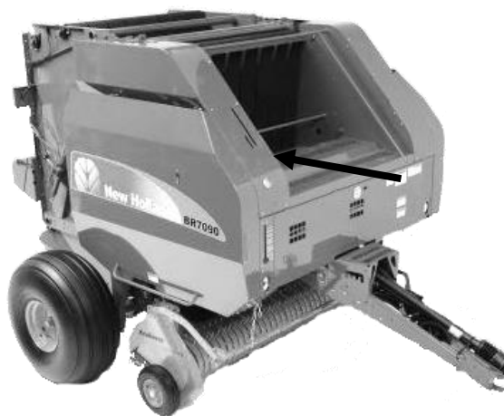
Mount THS on Left Side of Bale Chamber Panel Above Baler Shelf
