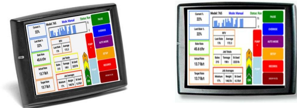
The 700 series integration to the Baler VT allows for the ability to set your real time baling through the baler VT and monitor both baler settings and Harvest Tec system parameters on one screen to ensure the most precise application to every bale.
