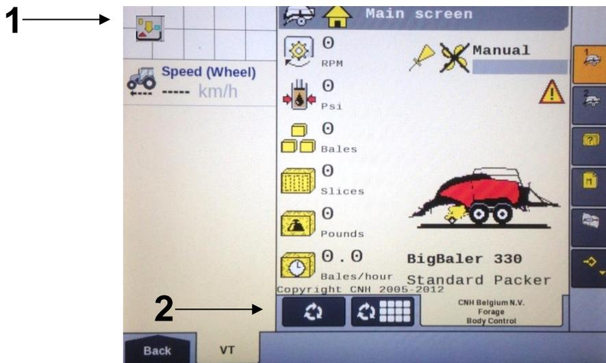
Once the object pools have been loaded and Icon (1) disappears from the upper left corner of the display, press the NEXT IMPLEMENT button (2) and verify that the 700 Series object pools appear on the Virtual Terminal.
