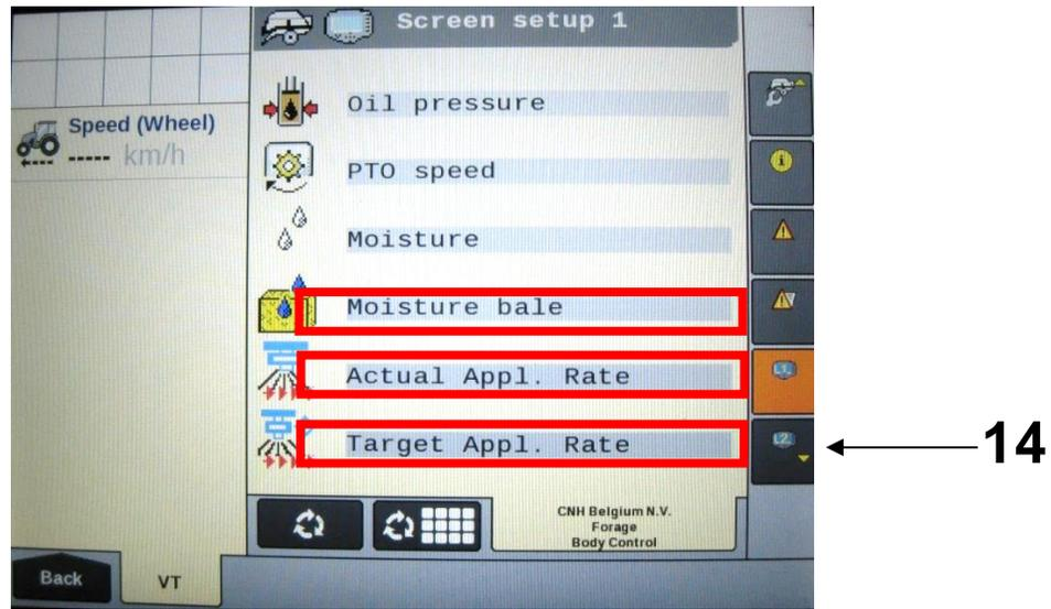
Selections related to the 700 series system include Moisture, Moisture Bale, Target Application rate, and Actual Application Rate, and are highlighted by arrows above and in the next picture. Scroll to additional options in the popup window by pressing the down arrow on the side of the popup window (15).
