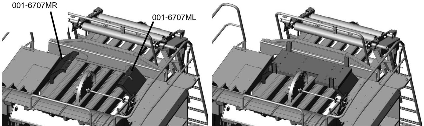
1. Install the two saddle legs (001-6707MR & 001-6707ML) on to the top of the baler chute as shown.
