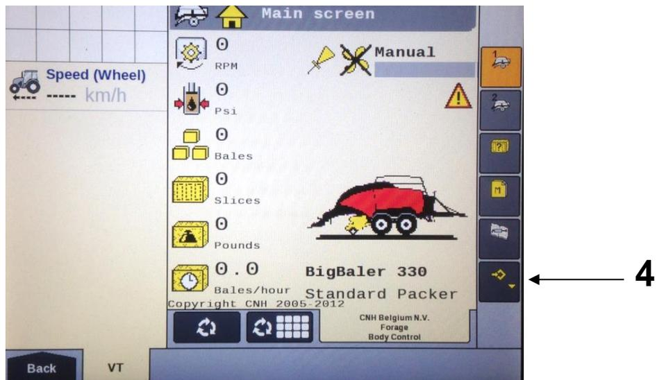
Scroll through the Menu bar until the INFORMATION icon (5) is visible. Press the INFORMATION button so the Information page appears. Verify that the controller software loaded to the baler is version 4.2.0.0 or higher. If not, contact the dealer to update firmware in Baler Control Module (BCM). If the controller software displays version 4.2.0.0 or higher proceed to configuring the baler for the 700 series system by pressing the MACHINE SETUP button (6).
