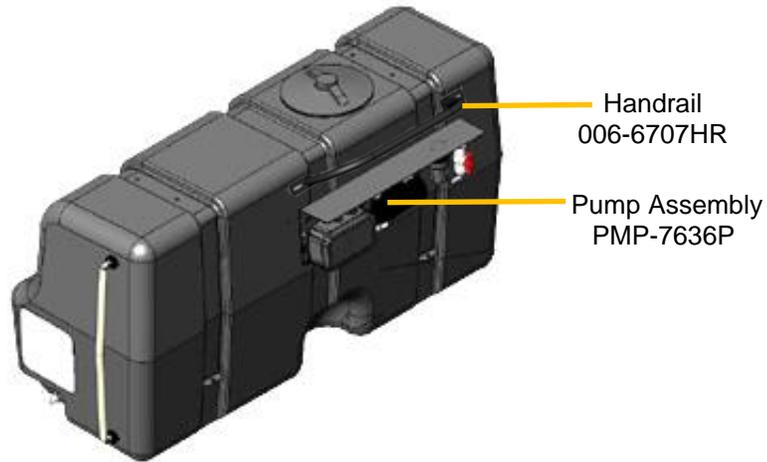
1. Attach handrail (001-6707HR) to tank with two 3/8" x 3/4" flange bolts.
