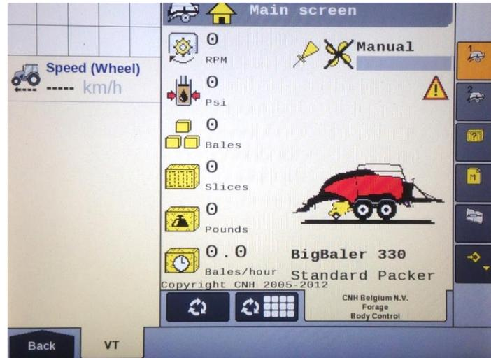
Icon (1) indicates that the object pools are in the process of loading and saving to the VT. Note that if the language selection of the VT is changed, the corresponding object pool must be reloaded to the VT. The object pool loading process takes approximately two minutes to complete.
