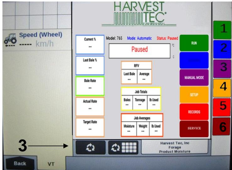
Press the bottom button of the Menu Bar with the down arrow in corner (4) on the side of the screen to continue down the Menu Bar below the USER SETTING icon.
