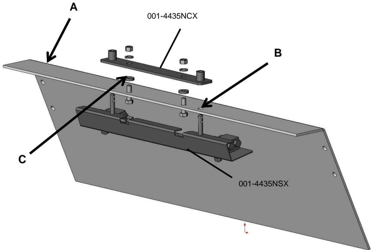
1. Locate the flat steel directly above the stuffer forks. **(A)**
