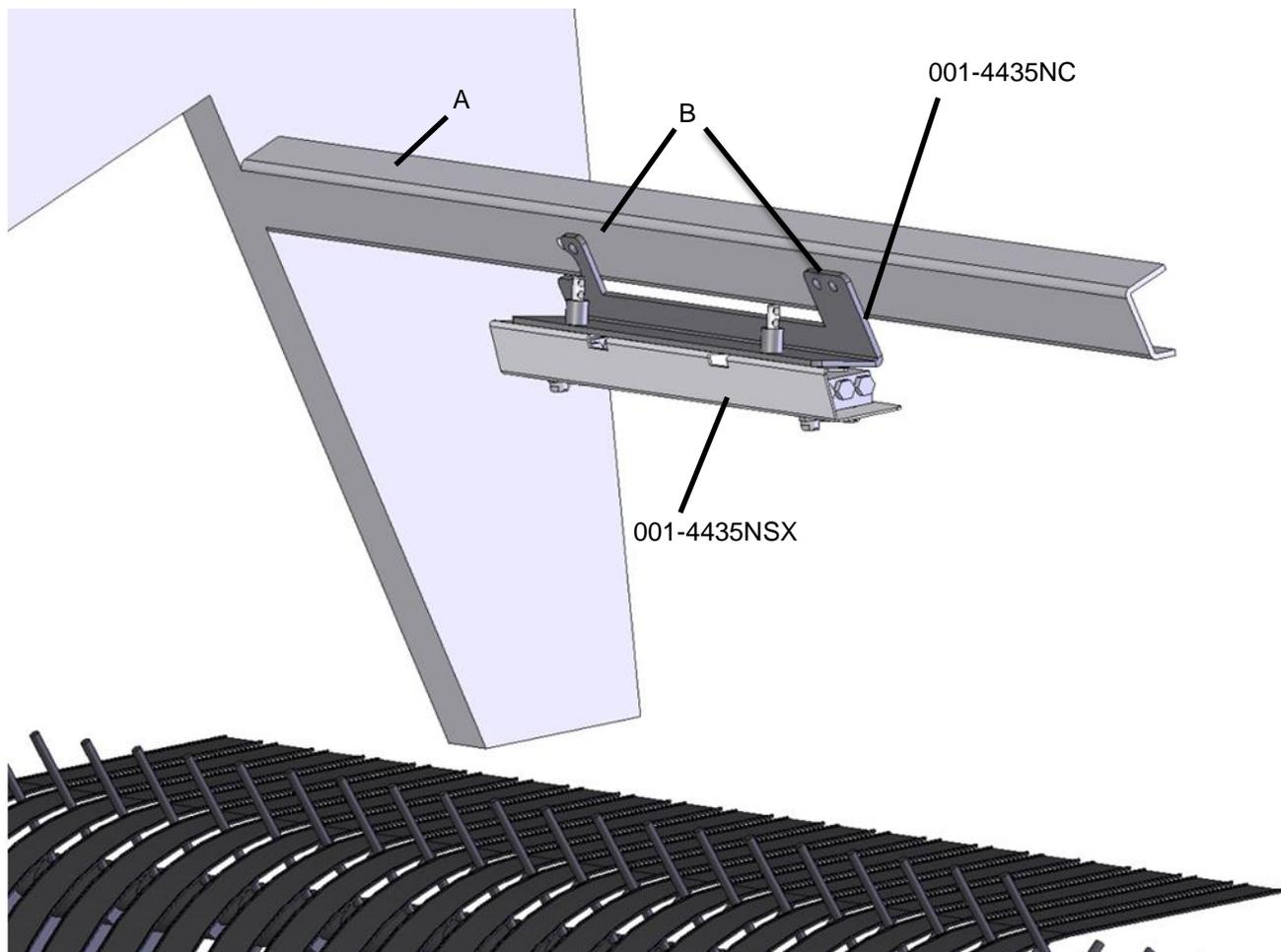
1. Locate the baler cross member directly above the rotor. **(A)**
