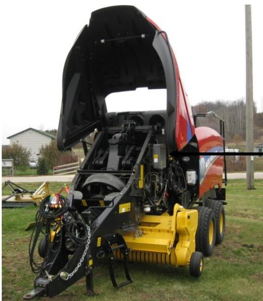
Locate the CAN port on the baler and attach baler ISO integration harness (006-765VA) to that location.
