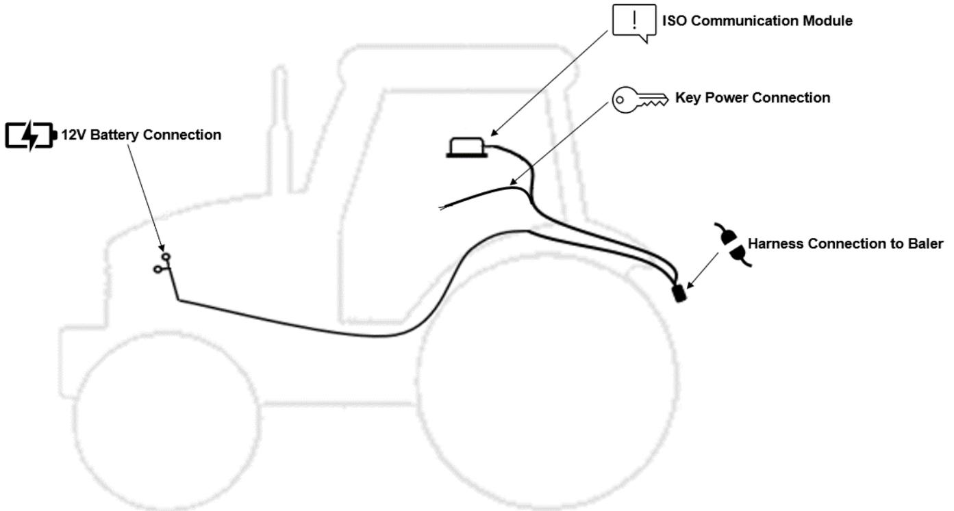
The general tractor setup of the 700 Series applicator can be seen above. The main harness of interest is the tractor power/communication harness (006-7651C). This harness will connect at the tractor battery, to the ISO Communication Module (ICM) mounted in the cab, a keyed power connection point, and connect at the hitch area to the baler power/communication harness (006-765B). View below to see highlighted installation instruction:
