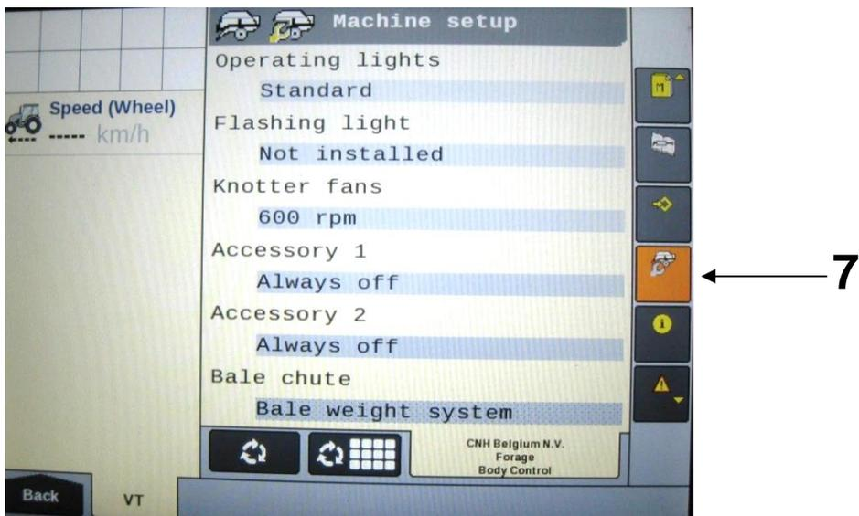
The second page of the Machine setup is identified by the three gray buttons in the Menu Bar. Press and hold the third gray button (8) for 10 seconds or until the display switches to displaying Dealer Mode.
