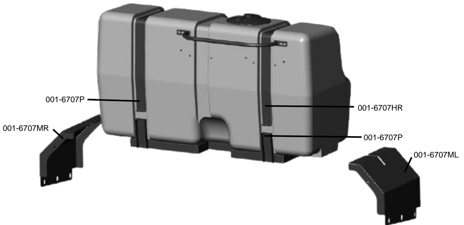
1. Remove the two tank straps (001-6707P) by removing all eight 3/8" hex nuts.
