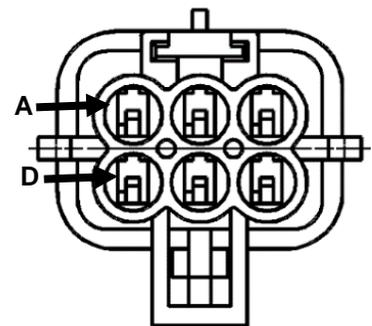
**Pump Connection on 700 Controller Harness**
