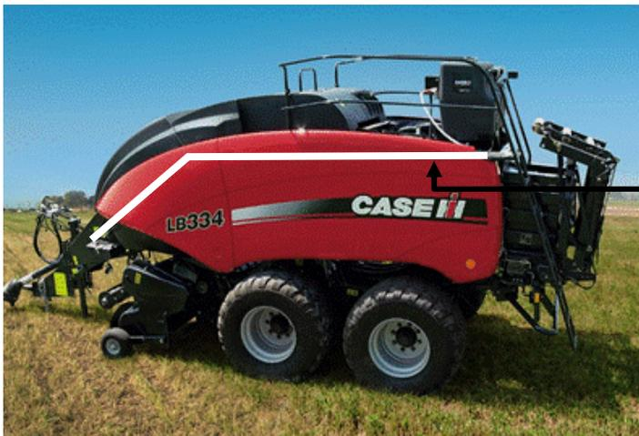
Route harness (006-765B) along inside of the baler. Keep harnesses away from moving parts and hydraulic hoses. Secure with existing cable clamps or use cable ties. When all connections are made to the IPM secure wires.
