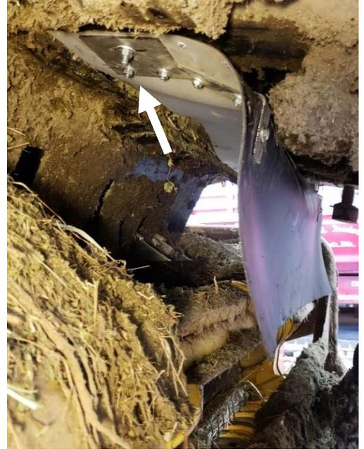
**Note: If installed correctly, the wind guard should not contact the fly wheel or center feed roll when the pick-up head is fully lifted.**
