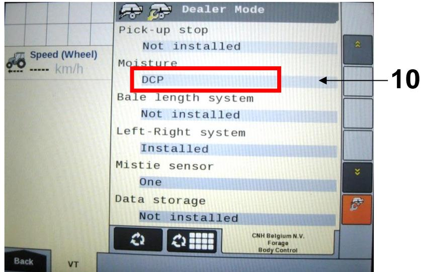
Select the proper configuration setting from the pop-up menu (11), based on the configuration of your 700 series system. This configuration setting allows the baler to properly display the information it is receiving from the 700 series system on the baler working screen. Select "DCP."
