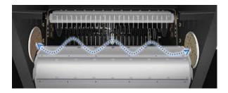
The H2O moisture sensor has two star wheels or discs in the bale chamber that read across the width of the bale. Taking 5 readings of resistance per second, giving the operator complete visibility of crop conditions.
