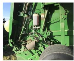
The Dye Marker Accessory consists of a tank, pump, end of bale sensor kit (200FCA), harness, and mounts on the baler. The spray option can be activated by selecting the feature in the H2O App and simply setting the moisture threshold you want to identify.
