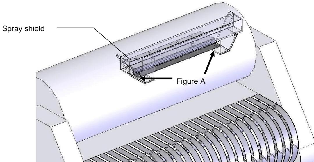
Locate the two bolts show in Figure A. Remove bolts and install spray shield holder (001-4435EK). Install bolts and tighten. Install spray shield assembly (001-4435ES) and secure with two supplied lynch pins. Use the inside slots on 3x3 balers and the outside slots on 3x4 balers.
