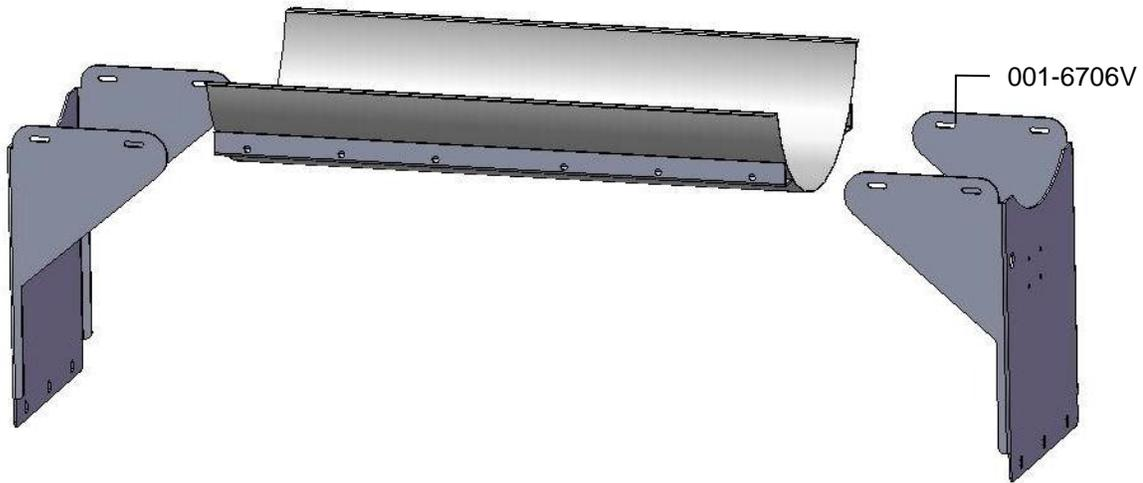
1. Locate parts bag 3. Install both saddle legs (001-6706V) onto the saddle (001-6706A) with eight 3/8" x 1-1/4" bolts, locks, and flat washers. Note: For 3 x 3 balers the slots in the legs will attach to the second and fourth weld nuts in from each end, of the saddle, on both sides. For 3 x 4 or 4 x 4 balers the slots in the legs will attach to the first and second weld nuts in from each end, of the saddle, on both sides.
