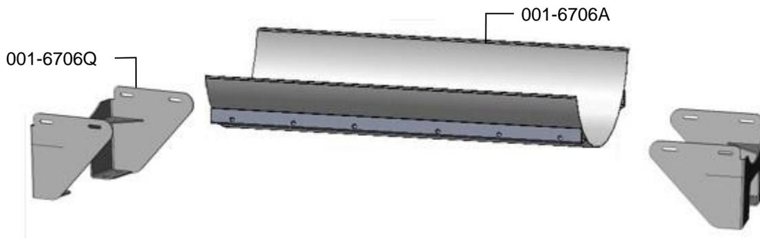
1. Locate parts bag 21. Install both saddle legs (001-6706Q) onto the saddle (001-6706A) with six 3/8" x 1-1/4" bolts, locks and flat washers. The mounting slots in the legs will attach to the second and third weld nuts in from each end, of the saddle, on both sides.
