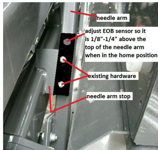
The end of bale (EOB) sensor mounts in the EOB bracket (001-4648C) as shown in the picture. The EOB bracket is mounted to the top side of the needle arm stop using the existing hardware that secures the bumper to the stop.
