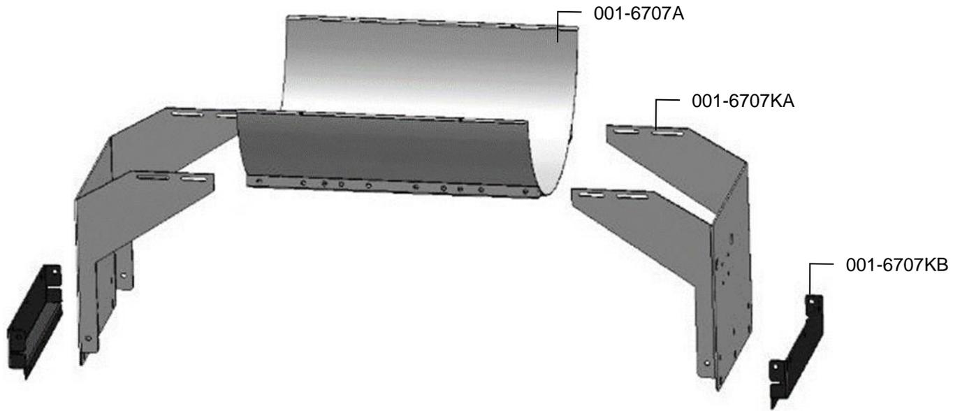
1. Locate parts bag 3. Install both saddle legs (001-6707KA) onto the saddle (001-6707A) with eight 3/8 x 1 1/4" Bolts, locks and flat washers. The mounting slots in the legs will attach to the first and second weld nuts in from each end, of the saddle, on both sides. \*Install leg extensions 001-6707KB if the baler was manufactured after 2010. Pre-2010 models do not need the extensions.
