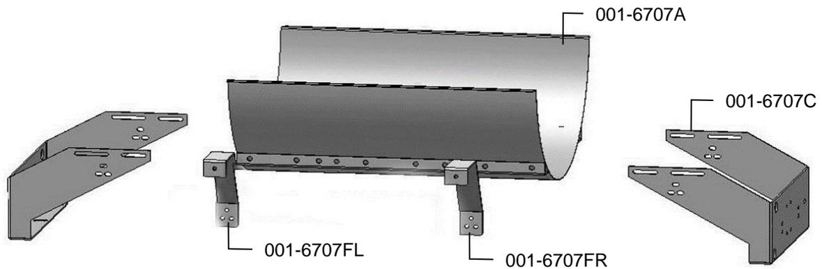
1. Locate parts bag 2. Install both saddle legs (001-6707C) onto the saddle (001-6707A) with eight 3/8" x 1-1/4" bolts, locks, and flat washers. Note: For 3 x 3 balers the slots in the legs will attach to the second and fourth weld nuts in from each end, of the saddle, on both sides. For 3 x 4 or 4 x 4 balers the slots in the legs will attach to the first and second weld nuts in from each end, of the saddle, on both sides.
