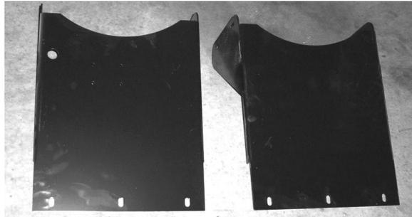
\*If the applicator is being mounted on a **Krone 870 HDP** baler, two leg adapter brackets will be needed for proper tank leg installation (below). Part number 001-6707KV.
