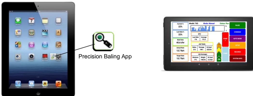
The iOS or Android Tablet displays offer the ability to communicate with the 700 series applicator system via hard-wired connection to the ISO Communication Module (ICM). Through the free Precision Baling App, the operator can set real time baling parameters to ensure the most precise application to every bale.
