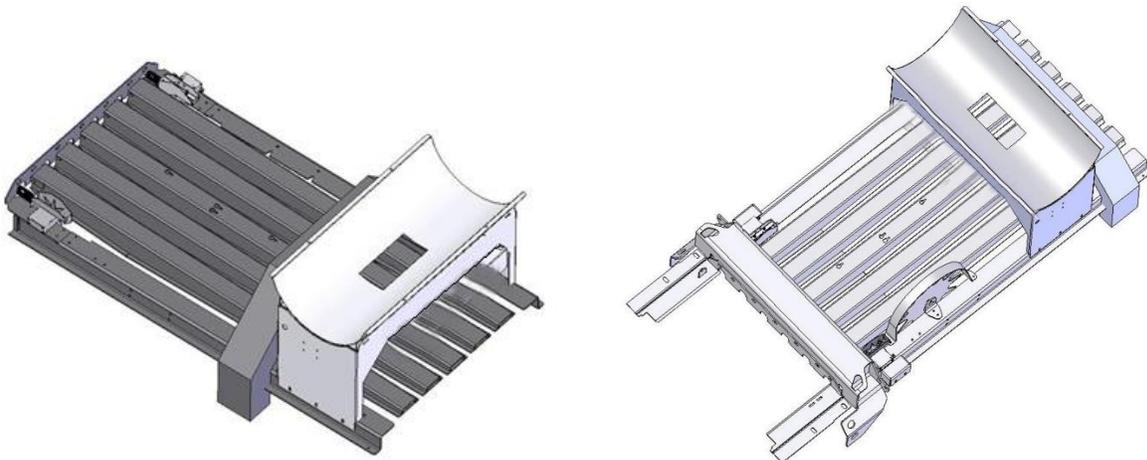
\*If the applicator is being mounted onto a **Krone 870 HDP, 1270, or 1290 HighSpeed** baler, two leg adapter brackets will be needed for proper tank leg installation. Part number 001-6707KV as seen in the image to the right.
