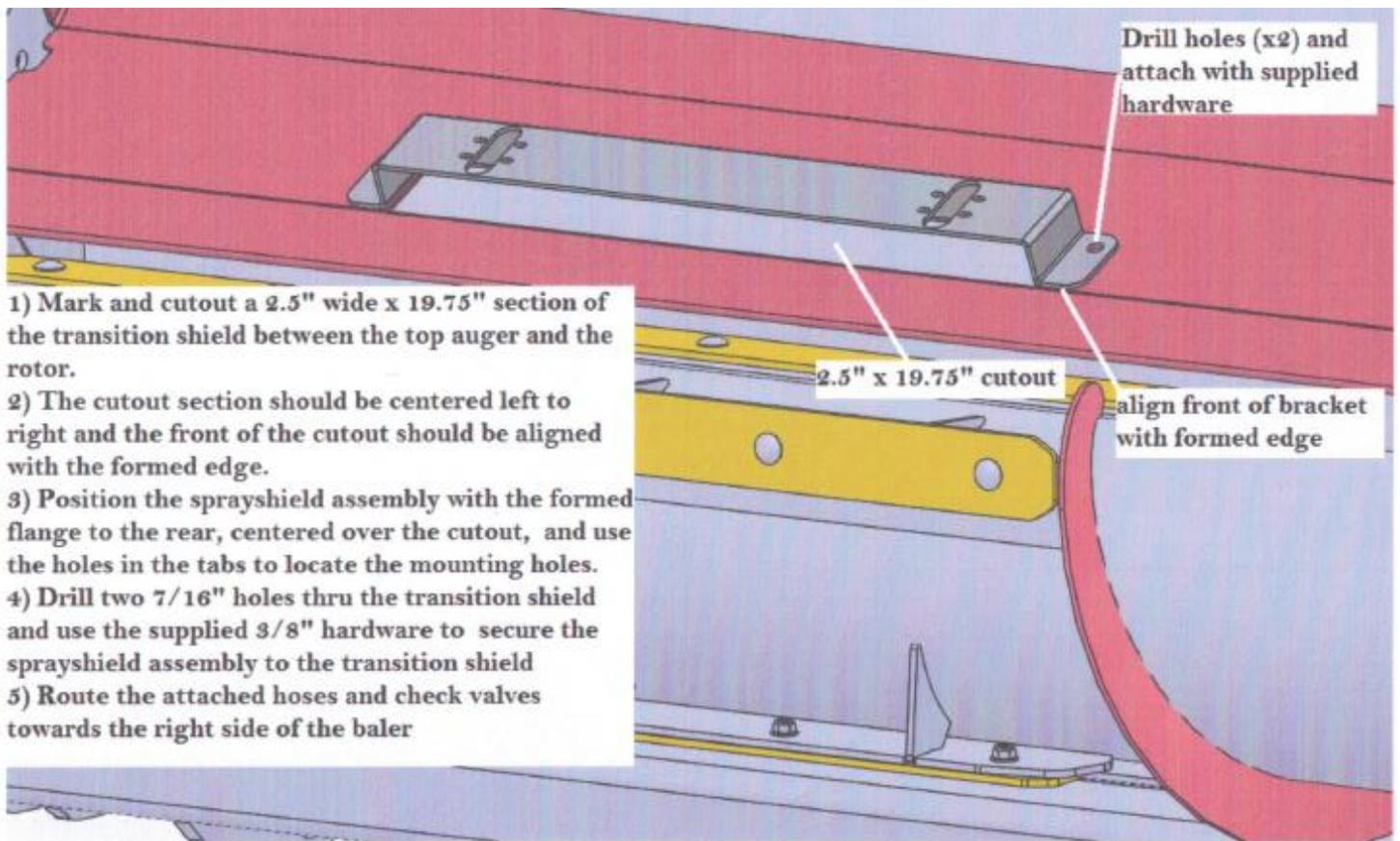
Locate nozzle bracket 001-4435NKS. Center the bracket on the top of the rotor shield and aligned with formed edge. Mark and cut out a 2 1/2" x 19 3/4" (64mm x 47cm) section of the transition shield between the top auger and the rotor. The cutout section should be centered left to right and the front of the cutout should be aligned with the formed edge.
