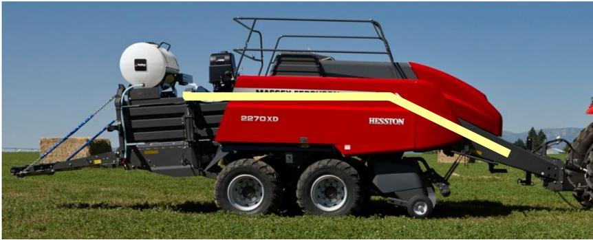
Route harness 006-765B or 006-765B2 along this path or similar on top of or inside of the baler from the pump plate to the hitch of the baler. Note: the end of the harness that has the large plug with sockets and the white heat shrink label, will be at the hitch of the baler. The other end attaches to plug on pump plate. Keep harnesses away from moving parts and hydraulic hoses.
