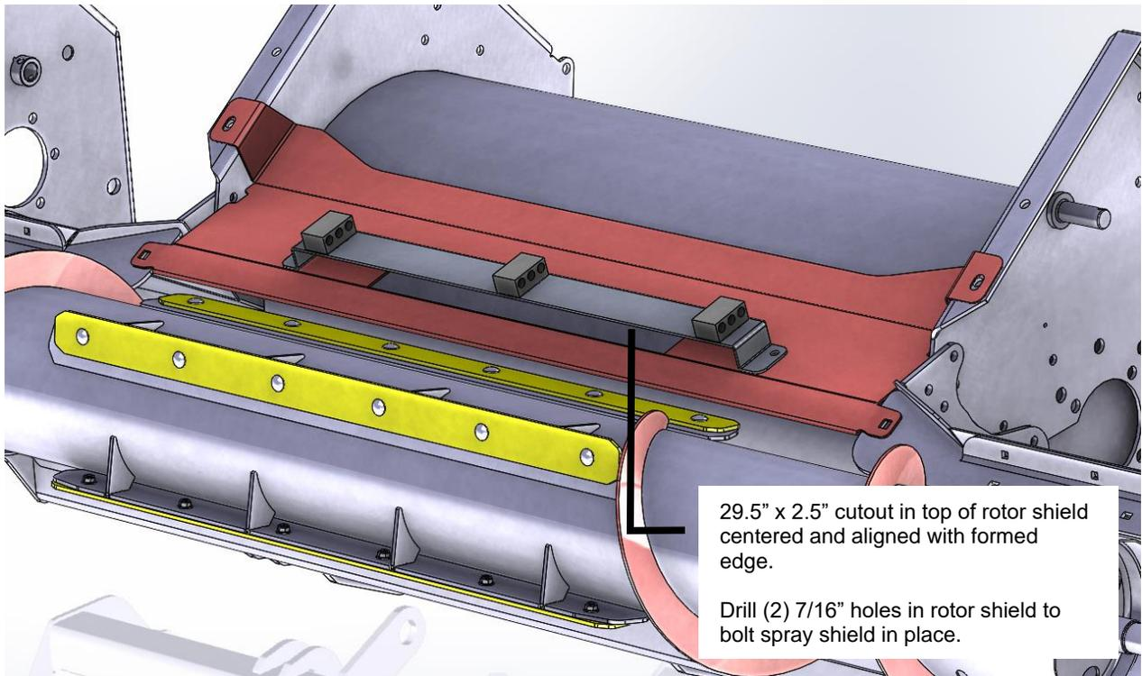
Locate nozzle bracket 001-4435NK. Center the bracket on the top of the rotor shield and aligned with formed edge. Mark and cut out a 2 1/2" x 19 3/4" (64mm x 47cm) section of the transition shield between the top auger and the rotor. The cutout section should be centered left to right and the front of the cutout should be aligned with the formed edge.
