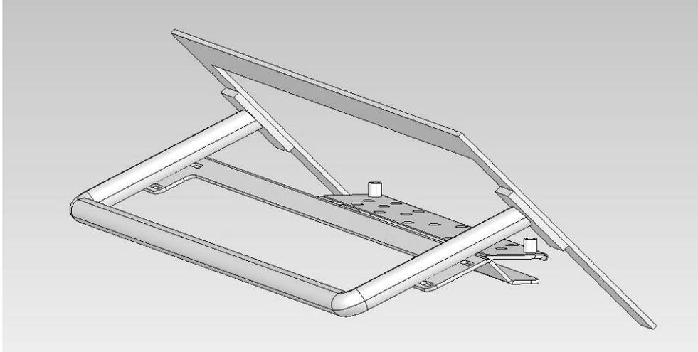
Locate the curved tube above the auger and rotary cutting system. Attach Shield holder (001-4440A) using the four supplied U-bolts, nuts, flat and lock washers. Slide shield back as far as the baler will allow and tighten down all mounting hardware. Install spray shield (001-4810) and use the two lynch pins (008-4576) to secure. A parts breakdown of the 4509C install kit is shown in the back of this manual.
