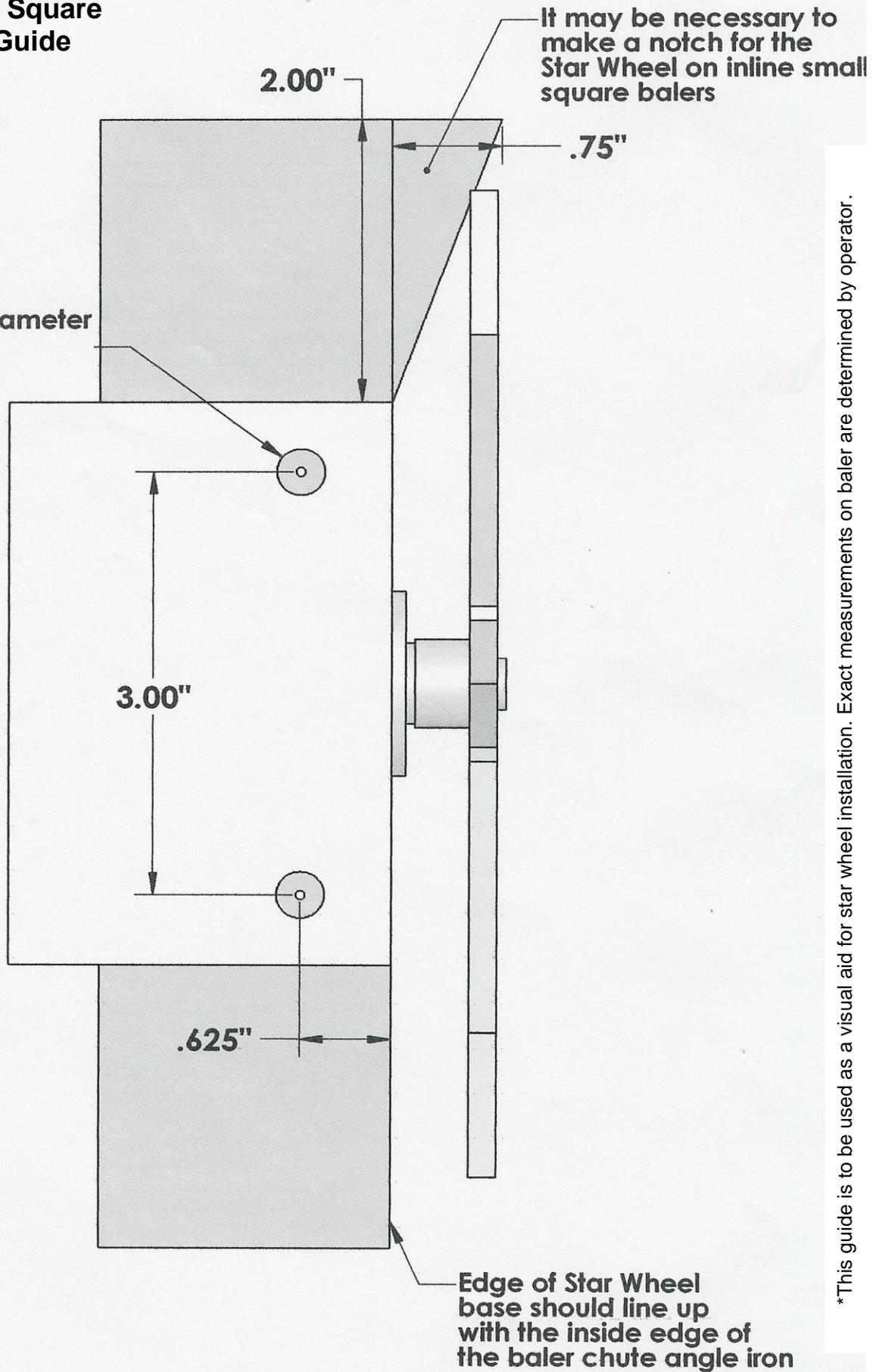
\*This guide is to be used as a visual aid for star wheel installation. Exact measurements on baler are determined by operator.
