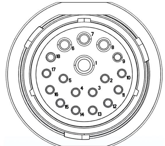
\*IPM Module Whip Plug- Pin # 5 Not Used
