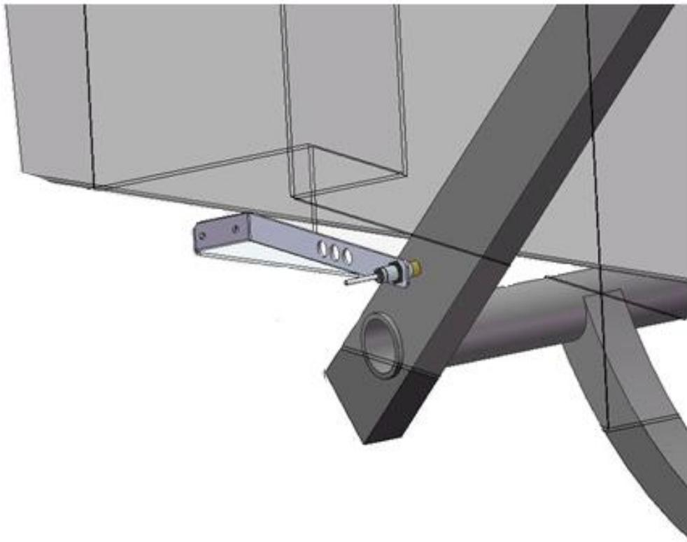
Mount the end of bale sensor bracket (001-4648) as shown. Mark and drill two 3/8" holes and attach the bracket using two 5/16" x 1" self-tapping screws, and 5/16" flange nuts. Mount the sensor in a hole location centered over the needle arm, keep the sensor 1/4" (7mm) from the needle and tighten both nuts. Run the sensor cable up to the main harness (006-765B2) and attach to port labeled EOB.
