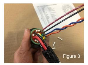
3. The GPS expansion harness (006-765GPS-EXT) has a 3 Pin triangular plug with 3 wires leads terminated with socket connectors. Install the socket connectors by identifying each colored wire on the GPS expansion Harness and pushing them into the corresponding open cavity in the back side of the 18 Pin connector (Figure 3). Reference wire pinout "Power / Communication Harness 006-765IC at Baler Hitch" in pin out section and the chart below to locate wire color with corresponding plug pin #.
