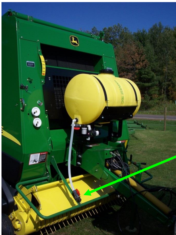
Drain/Fill line on the baler
