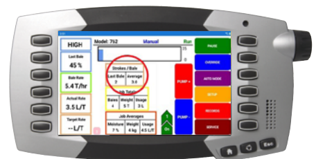
Hayboss 700 series can be displayed thru a dedicated ISOBUS terminal with the addition of optional adapter harness
