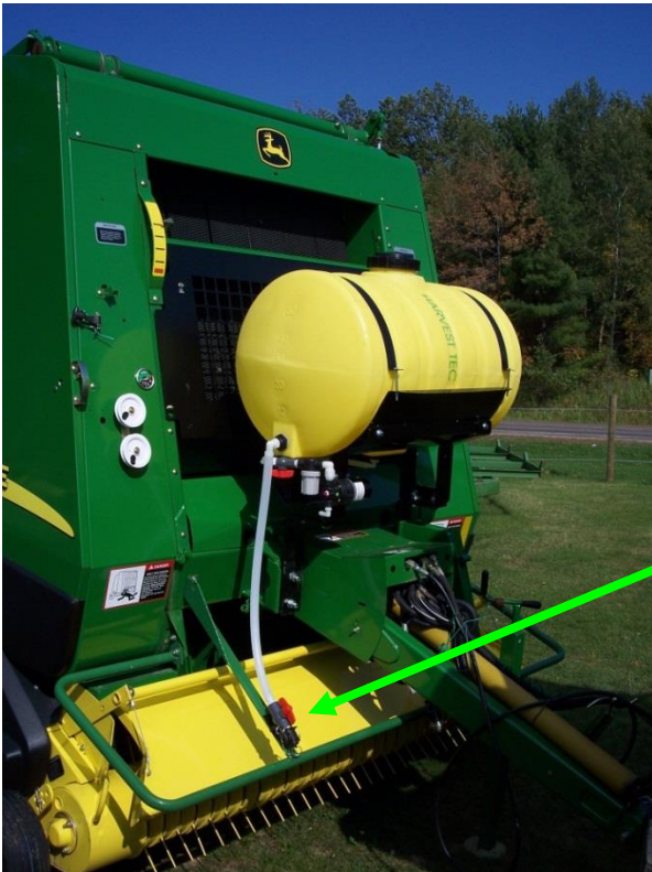
Drain/Fill line on the baler
