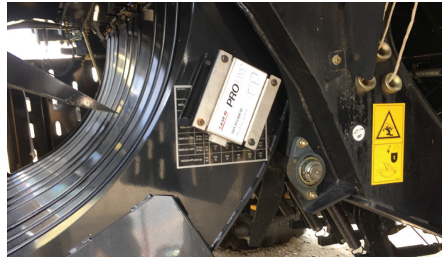
▲ Pre-compression chamber mounting location
