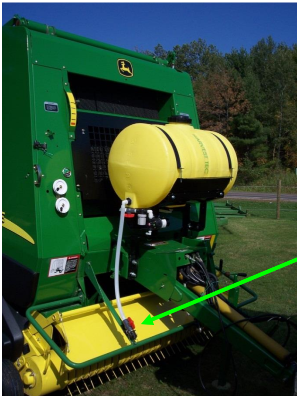
Drain/Fill line on the baler
