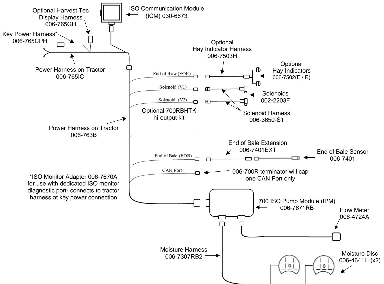
\*ISO Monitor Adapter 006-7670A for use with dedicated ISO monitor diagnostic port- connects to tractor harness at key power connection
