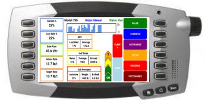
For those operators who have a dedicated ISO display with in cab harness diagnostic port connection, the 700 series can populate as its own object pool. Adapter/integration harness 006-7670A (sold separately) is required for connection. This adapter/integration harness supplies key power and communication thru ISO diagnostic plug found in cab.
