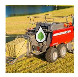
The optional HT238DM Dye Marker Accessory can be added to the HT200A2 kit that will mark every bale that is above a set moisture with a red, food-grade stripe.
