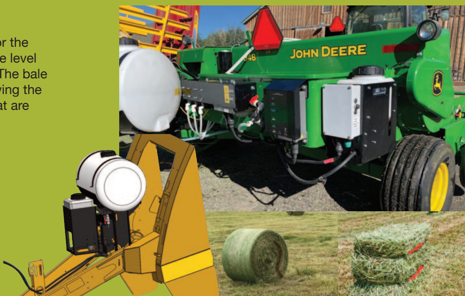
A food-grade stripe is applied to indicate higher moisture areas of the bale using the optional Dye Marker kits available for both Round and Small Square balers.
