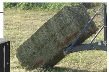
The system sprays red, food-grade dye on the bales when the moisture is above your set limit.
