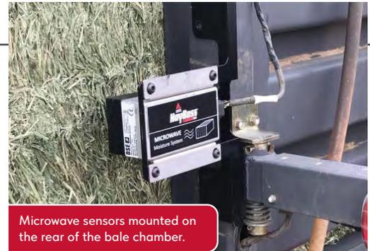
Microwave sensors mounted on the rear of the bale chamber.
