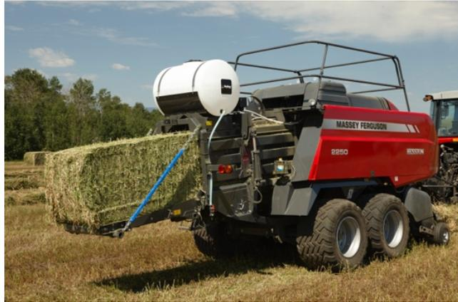
For contractors and other baler users, this has the great benefit that when applied at the correct rate, by enabling hay to be safely baled at above 15% moisture, this offers the potential to lengthen the baling day by maybe an hour each end or bale on days when previously the crop would not be dry enough.
