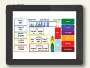
If a baler or tractor is not equipped with an ISOBUS monitor, the operator also has the option of using their own tablet display via charging cable into the ISO Communication Module located in cab of tractor. Any one of these options give the operator complete control and provides information for any baler equipped with the automatic applicator. The baler monitor and tablet display:
