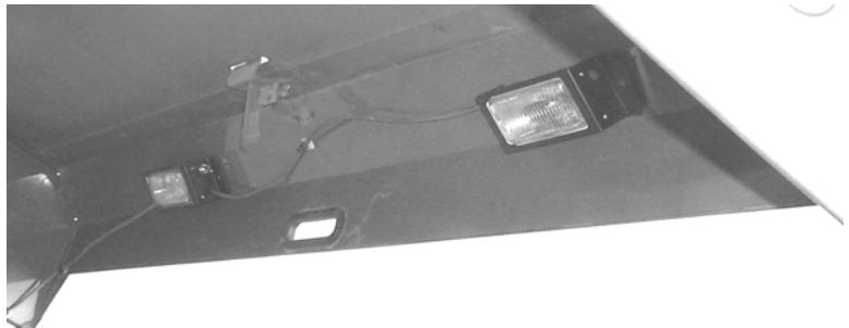
STEP 2: Spread the lights apart so they are 14 inches from each side of the edge of the surface wrap compartment. The lights should fit between the two spots where the compartment comes in contact with its stops on the bottom of the frame. These areas should be marked to assure that the lights don't come in contact with the stops when closing the compartment.
