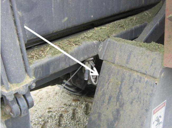
Locate the communication harness (006-5650J) and locate the connection point shown below on the baler. The connection point is shown to the right by the arrow. This location is at the back of the baler behind the right fender. Remove the cap and connect the communication harness (006-5650J). Route the harness over the fender and up the twine box towards the PIP on the back right twine box. Secure loose wires with cable ties.
