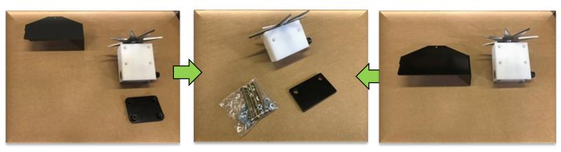
Setups with **grey** twine diverter will use the black filler plate with new style star wheels.
